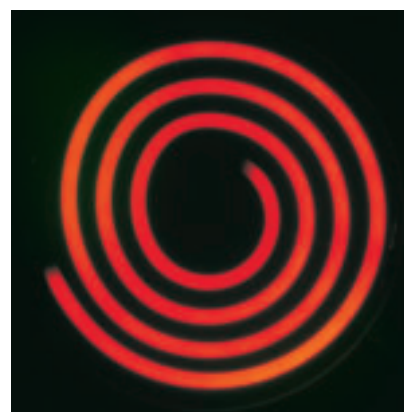
Figure 6 Electrical energy is transformed into thermal energy in the metal heating coil. As the metal becomes hotter, it emits more radiant energy.
