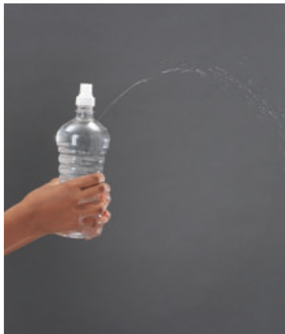
Figure 20 When you squeeze the bottle, the pressure you apply is distributed throughout the fluid, forcing the water out the hole.
